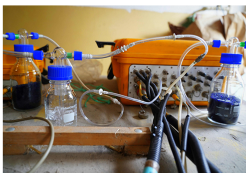
Figure 1. LI-COR LI-7810 Automatic CO 2 , CH 4 and H 2 O Analyzer with LI-8250 Multiplexer
